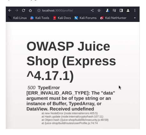
Bad error handling should return custom page with no sensitive information what is went wrong. Returning used node modules and information about how the web application is working.
