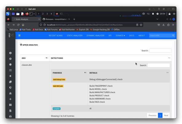
This section can be particularly beneficial when concentrating on binary analysis, especially in the context of malware. For instance, when running the application on an emulator, it may be discovered that the malware includes anti-VM code, altering the application's behavior in the emulated environment.
