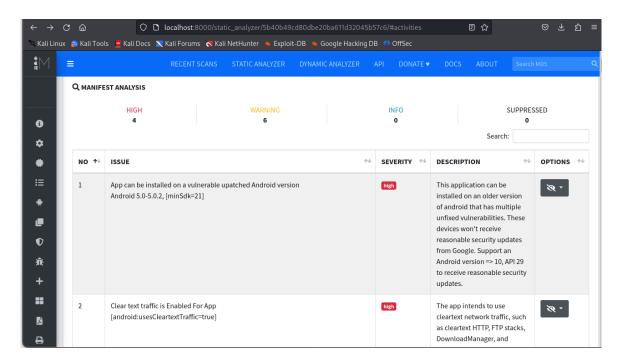
Code analysis - This section can provide clues that may help uncover additional exploits. It has been identified that the application logs sensitive information. We can also investigate where exactly such information can be found using the provided binary paths. Another issue pertains to the fact that information is being stored in external memory that can be browsed by other applications, potentially leading to leaks of sensitive information.
