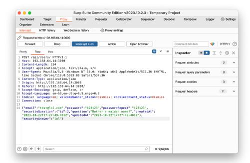
Server is not checking if data filled in request are valid so we can create a lot of dummy accounts with not valid emails, short passwords etc. It is even possible to send empty Json file and create infinity dummy accounts which can result in filling up the database and decreasing application performance. Example below:
